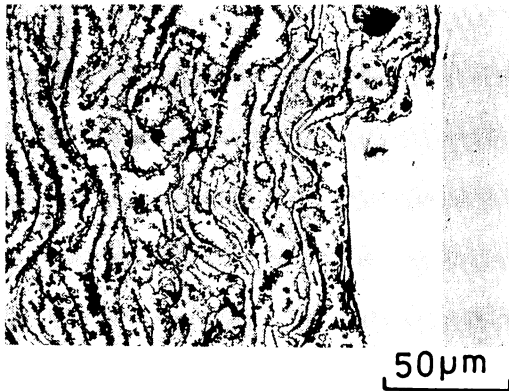
Photo 7 Structure of thermal-sprayed coating layer of Fe-4.5%C alloy after holding at 900°C for 3hr.
